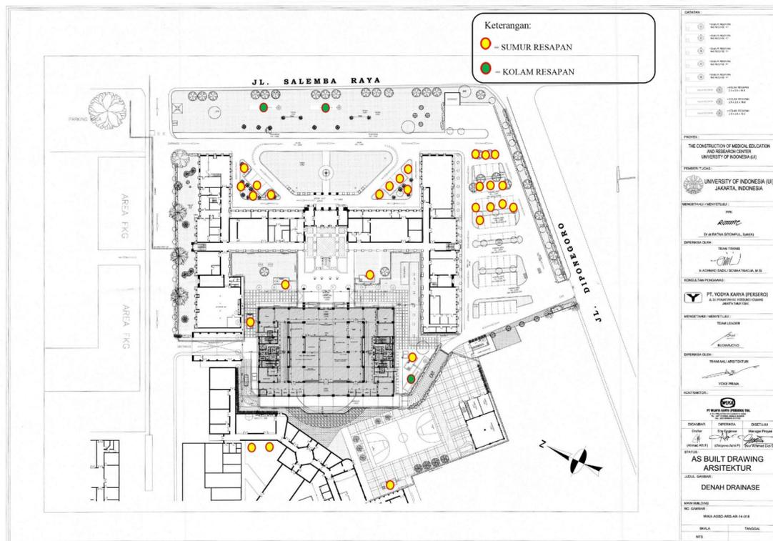
**Layout of Infiltration Wells/Retention Ponds at Salemba**
